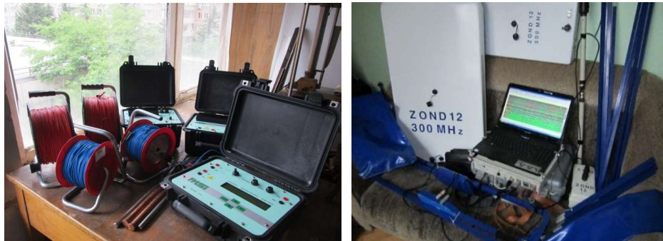
a. b. Fig.1. a) Earth Resistivity Meter PASI 16GL-N, b) ground penetrating radar ZOND 12
