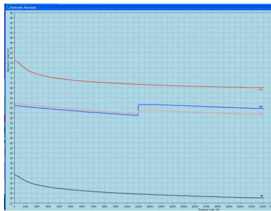
Fig.11. Pressure changes graphic by reinjection for 70 years period
